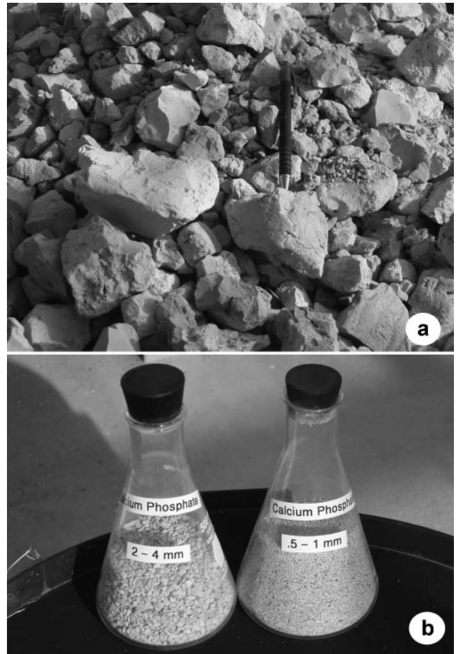
Fig. 1. (a) Recovered calcium phosphate precipitate from full-scale wastewater treatment plant. (b) Selected particle sizes after grinding and sieving the recovered phosphate material.
